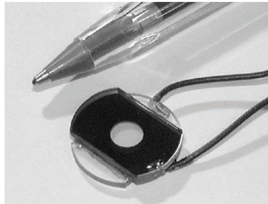
**Fig. 2:** Liquid crystal lens (photo from [2])
