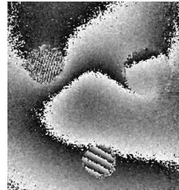
**Fig. 6:** Deformation difference between a master and a sample object by projecting the conjugated wave front of the master onto the sample object like shown in Fig. 1. b).
