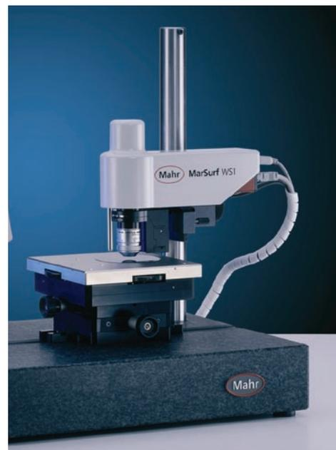
**Fig. 3:** Photo of the white light interferometer MarSurf WS 1
