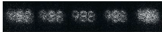
Fig. 2: Reconstructions of a diffusely transmitting object at 2 mm -interval reconstruction planes using multiple intensity measurements. The width of the whole object is 2 mm.
