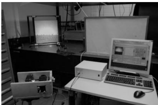
Fig 1: The photograph of the shearography prototype shows the main components: tripod mounted sensor head, electronics controller, PC and the laser. The object under investigation is a canvas painting sample from the TATE Gallery, London.
