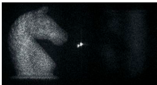
Fig. 2: Optical reconstruction of the recorded phase hologram with the display operated in phase-mostly mode.
