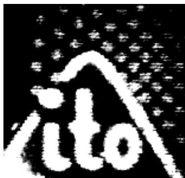
Fig. 2: ITO logo written into photo-addressable polymer.
