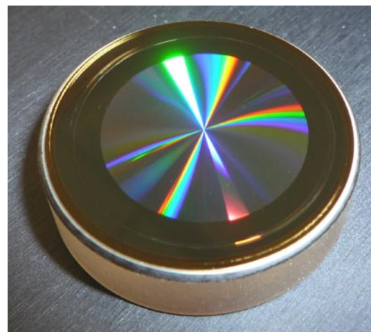
Fig 3: Photograph of an axicon-structure produced with scanning beam interference lithography.
