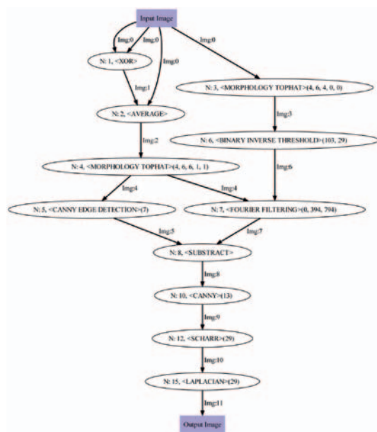
Fig. 5: Automatically generated algorithm for lens defect detection on microlens arrays measured using a confocal microscope with 20X magnification (see Fig. 4).
