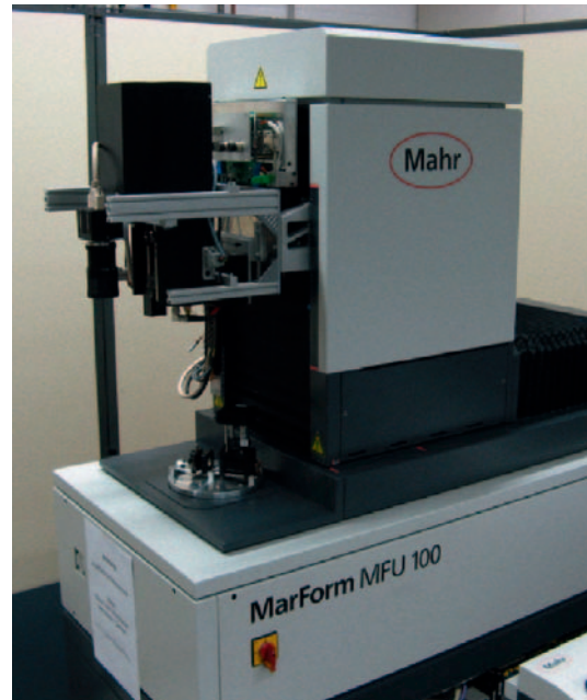
Fig. 2: Automated multi-scale measurement system based on a modified Mahr MFU 100.
