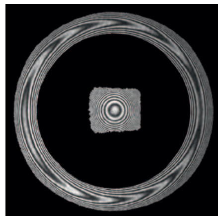
Fig. 2: Interferogram with the central point source activated.
