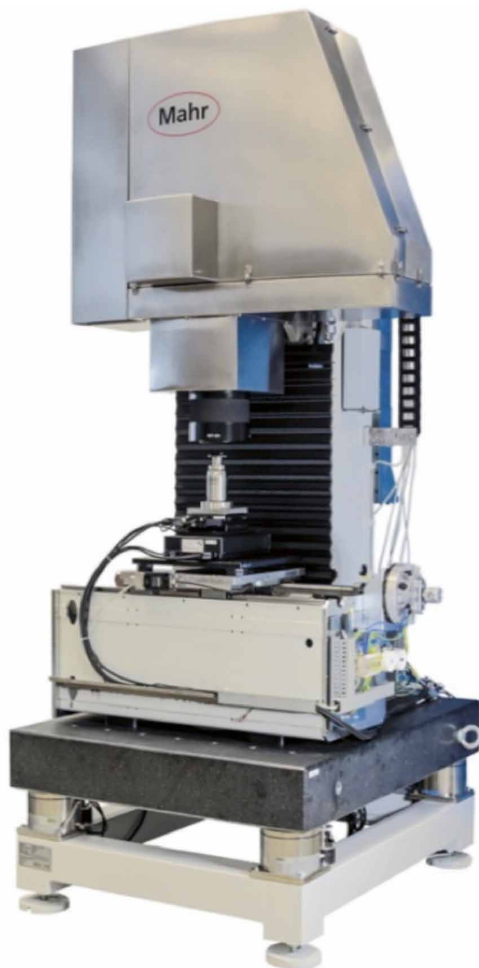
Fig. 3: Prototype of a Tilted-Wave-Interferometer built by the industry partner Mahr.
