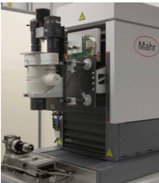
Fig. 1: Demonstrator setup for the inspection of small gear wheels based on a modified Mahr MFU 100 machine. The mounted sensors are a zoom fringe projection stereo microscope and a chromatic confocal point sensor.
