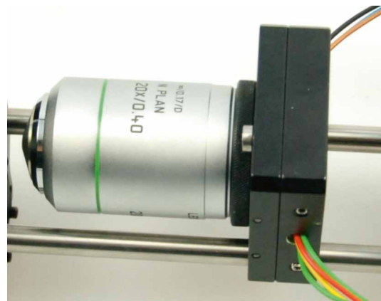
Fig. 2: Microscope objective with integrated AMiPola spatial polarization shaping system.
