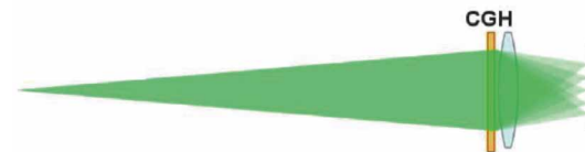
Fig. 2: Principle of holographic multipoint generation.
