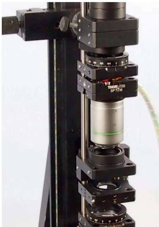
Fig. 1: Microscope with objective integrated spatial polarization shaping system.
