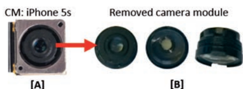
Fig. 2: Complete camera module of iPhone 5s [A] and different views of the removed optical module from the iPhone 5s [B].
