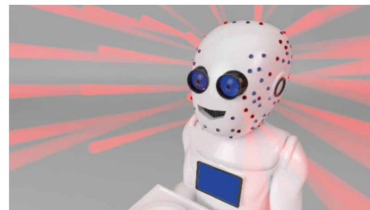
Fig. 1: Concept image of a service robot incorporating the Multi-Stereo Multi-Projection modules. The laser holographic point-cloud projections are displayed in red; the cameras are blue dots on the head.
