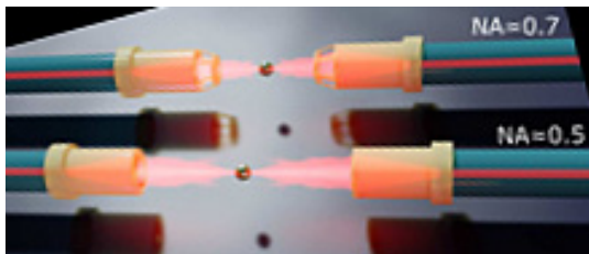
Fig. 1: Concept rendering of the optical trapping setup in a counter-propagation manner. DOEs control distance and trapping force. Image from [1].
