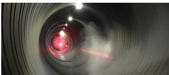
Fig. 1: View inside the fog chamber; fog is entering through multiple inlets along the bottom of the chamber, the beam of the HeNe-Laser is scattered by the fog droplets.
