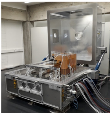
Fig. 1: The NPMM-200 at ITO. Machine in the opened vacuum chamber for thermal isolation. The measurement frame is made of ZERODUR.
