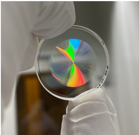
Fig. 1 Photo of a fabricated grating waveguide mirror.
