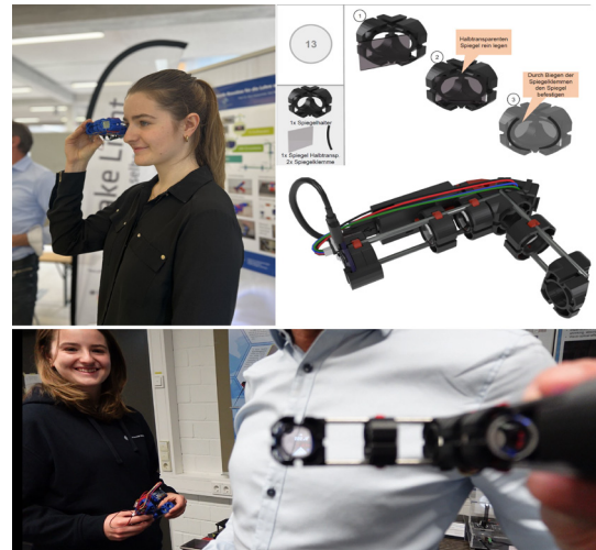
Fig. 1 GPS-based optical data glasses: demonstrator in operation and mechanical design.
