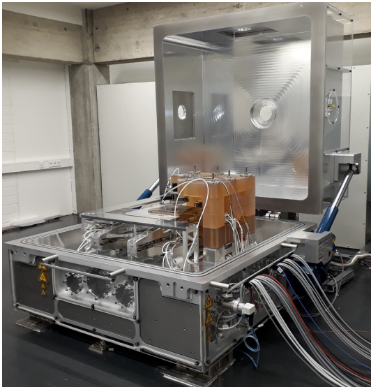
Fig. 1 The NPMM-200 at ITO. Machine in the opened vacuum chamber for thermal isolation. The metrological frame is made of ZERODUR.
