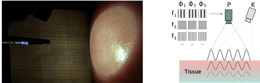
Abbildung 2: Left: Fringe projection onto tissue using the miniaturized fringe projector (V. Aslani), Right: SFDI principle
